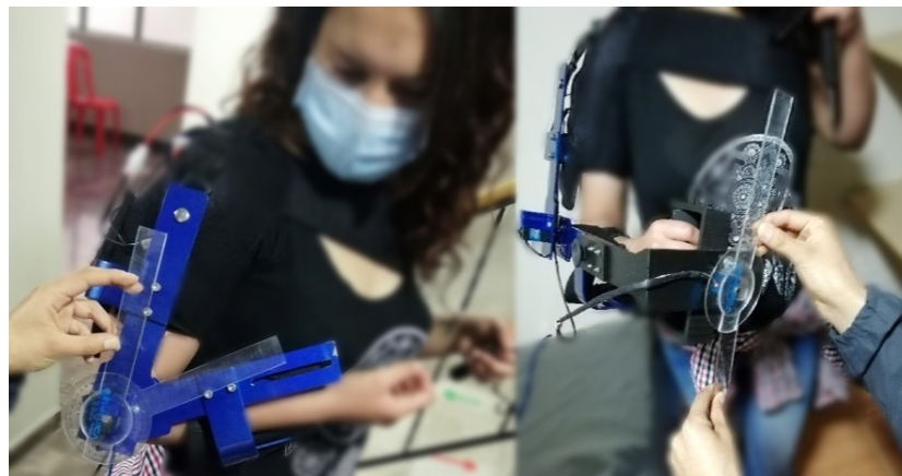
Figure 9. Prototype orthosis to support upper torso rehabilitation in case study.
