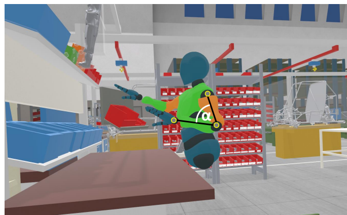
Figure 1. An avatar which performs movements at a virtual workplace. An exemplary representation of the relevant joint positions for the determination of the joint angle of the elbow flexion.
