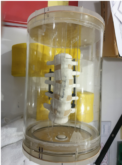
Figure 3 Experimental construct of lumbar spine model instrumented with carbon fiber/polyetheretherketone pedicle screws. Four pedicle screws (CarboClear™, CarboFix Orthopedics, Herzliya, IL, USA) were inserted into the left pedicles and two pedicle screws were inserted into the right pedicles, and connected by two longitudinal rods. The model was suspended on plastic rods and immersed in water.
