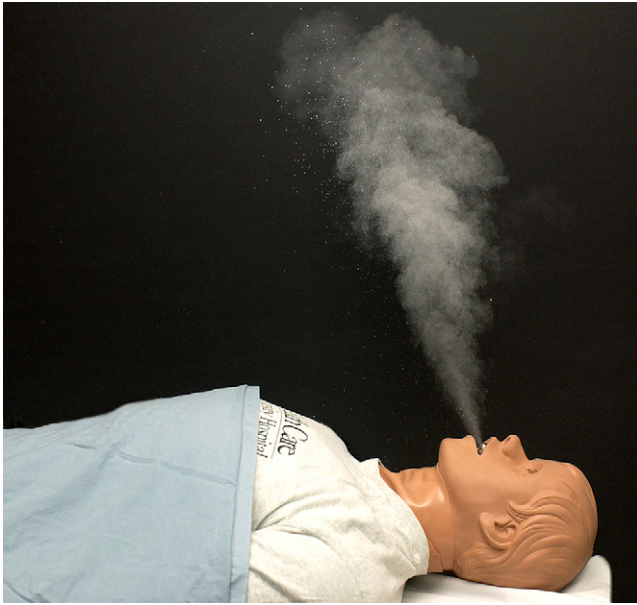
Fig 1. Visual demonstration of respiratory particle dispersal during cough using biosimulation and fluorescent powder.
