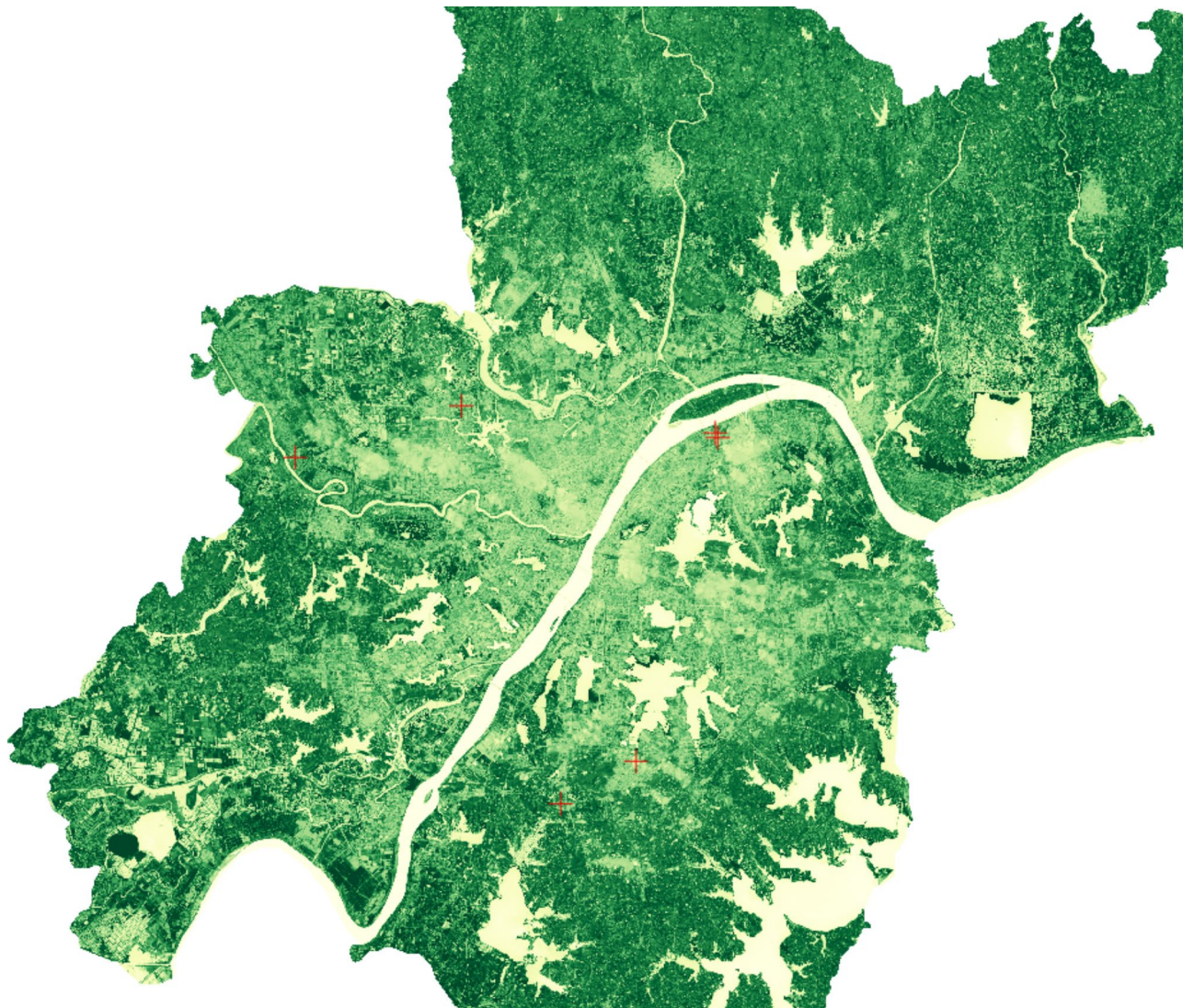
Fig. 3. The NDVI map of Wuhan. The remote sensing images of Wuhan were obtained using Landsat 8 satellite data, accessible via USGS Earth Explorer ( https://earthexplorer.usgs.gov/ ). The Normalized Difference Vegetation Index (NDVI) values, ranging from 0 to 1, were calculated using QGIS software ( https://qgis.org/en/site/forusers/download.html , version 3.34.8), to assess vegetation coverage in the region. Data processing and visualization followed standard protocols for remote sensing analysis.
