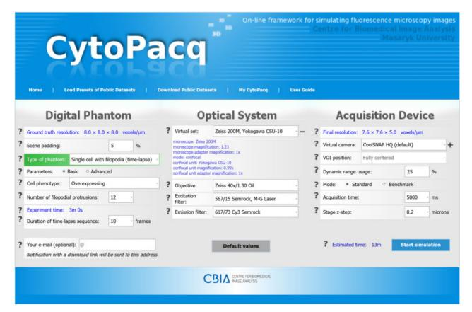
Fig. 1. A screenshot of the CytoPacq web-interface. The configuration form is divided into three sections, corresponding to the underlying simulation modules
