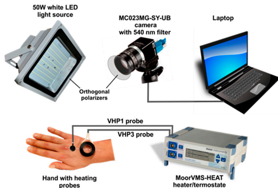
Figure 1. Remote photoplethysmography setup and used equipment; Palm dorsal aspect middle line is denoted by white dotted line.
