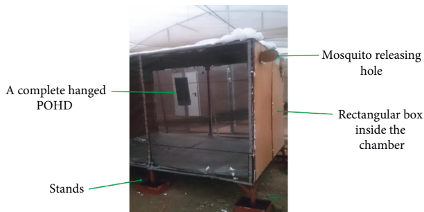
FIGURE 4: A bioassay box (187 × 212 × 115 cm) evaluating efficacy of POHD placed in the middle of a semifield chamber. The POHD is incorporated with different formulations of different synthetic attractive blends of different storage and usage period.
