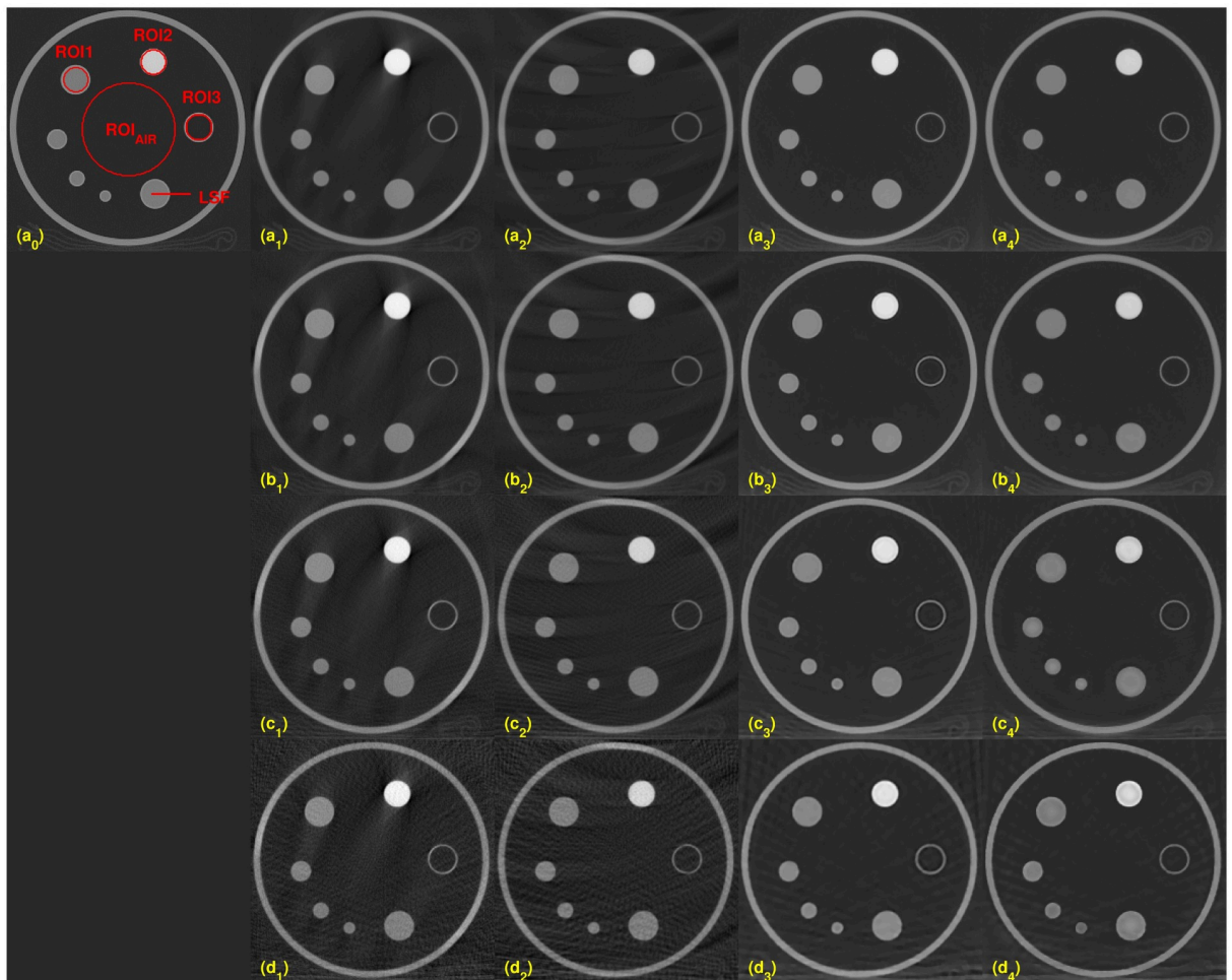
Fig 6. Reconstructed images with various sampling step sizes. From top to bottom, the sampling step size is set to 1, 4, 8, and 16. Each column consists of a different reconstruction algorithm, from left to right, scanner: FDK, Katsevich, TV and the TF algorithm. The image on (a 0 ) shows the three ROIs, and the red line is set for the computation of LSF for MTF. ROI AIR , ROI of air, is defined to compute the CNR for ROI1-ROI3.
