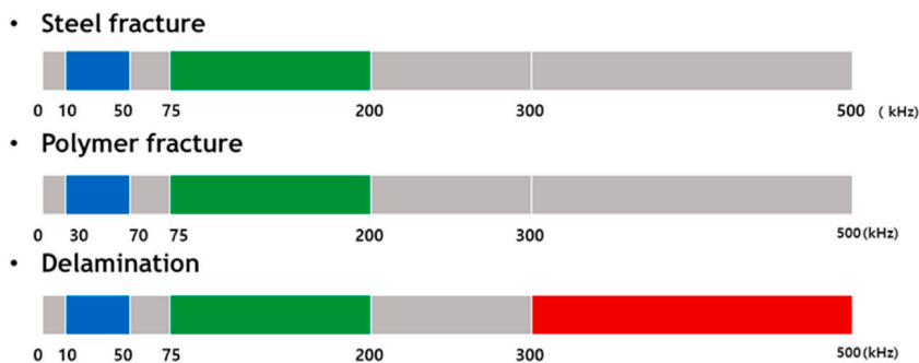
Fig. 8. Peak frequency bands of each failure mode for the steel–polymer sandwich composite. (color should be used). (For interpretation of the references to color in this figure legend, the reader is referred to the Web version of this article.)
