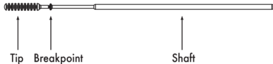
Figure S13. Developing a automation compatible swab. A major bottleneck in the sample processing is the manual process of opening tubes and removing the swab. Not only is this manual but also a source of both cross contamination and biohazardous exposure. To limit this, we designed a 3D printed swab, in conjunction with Applied Medical Company where the breakpoint was engineered to break close to the swab edge such that it would not interfere with our automated pipette machinery.
