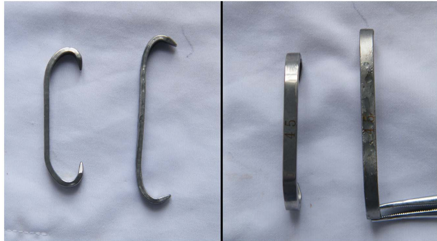
Figure 2. 45 mm Shape memory Alloy Hook (SMAH). Left, prototype; right, unfolded in ice and water mixture.
