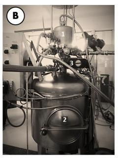
1: DIC Reactor 2: Vacuum Tank 3: Butterfly valve for Pressure Drop
