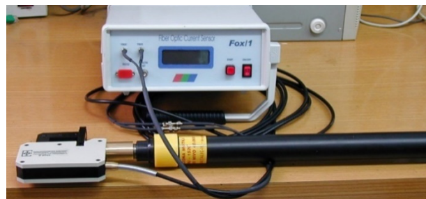
Figure 1. Portable OCT with measurement head mounted on an insulating rod certified to operate up to 100 kV.
