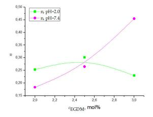
**Figure 7.** Dependence of *n* versus EGDM cross-linker content, according to p(NiPMAm) hydrogel swelling in fluid pH = 2.0 and pH = 7.4 at 20 °C.
