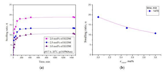
**Figure 6.** Swelling ratio,  $\alpha$ , of the poly(*N*-isopropylmethacrylamide) hydrogels at 20 °C and pH = 7.4 depending on: (**a**) time and (**b**) EGDM content.
