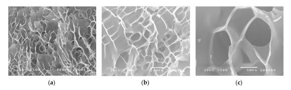
**Figure 3.** SEM micrographs of p(NiPMAm) hydrogel sample with 3.0 mol% of EGDM, swollen in the equilibrium state with magnification: (**a**)  $100 \times$  (scale bar  $100 \mu$ m), (**b**)  $200 \times$  (scale bar  $100 \mu$ m), and (**c**)  $500 \times$  (scale bar  $50 \mu$ m).
