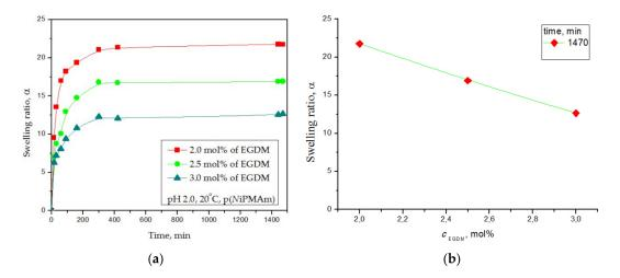
**Figure 5.** Swelling ratio,  $\alpha$ , of the poly(*N*-isopropylmethacrylamide) hydrogels at 20 °C and pH = 2.0 depending on (**a**) time and (**b**) EGDM content.
