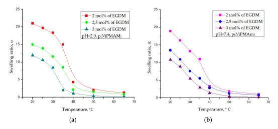
**Figure 8.** Swelling ratio,  $\alpha$ , for poly(*N*-isopropylmethacrylamide) hydrogels depending on the temperature in fluid with pH-values of (**a**) 2.0 and (**b**) 7.4.
