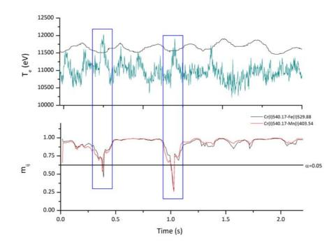
Figure 5 illustrates the electron temperature and correlation signals evolution in presence of variable welding speed. It is evident that instabilities in the molten pool as well as in the plasma plume are clearly detected by the sensor. In fact both the electron temperature and the correlation signal values exceed the threshold values.
