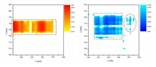
The measure of the correlation (anti-correlation) signal for a selected couple of lines allows to overcome the main drawback for the use of CMT in real-time sensors, that is the long acquisition and computation time requested for building the Covariance Map of the whole spectrum. By selecting only pairs of lines only a few number of the Covariance Matrix have to be evaluated paving the road towards the use of such a technique for real-time sensors [20].
