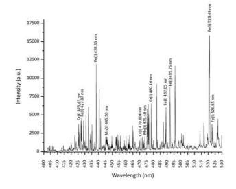
The measurement of the plasma electron temperature as well as the analysis of the plasma optical spectra by using the Covariance Mapping Technique have been the subject of several papers published by our research group over the last few years [17-20]. The final objective was to combine the two above mentioned techniques to develop an optical sensor for real-time defect recognition during industrial laser processes.
