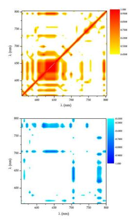
In Figure 2 two samples of the correlation and anti correlation maps in the case of laser welding of Al-Mg Aluminium alloy are shown. A positive correlation value between the intensity of emission coming from two different species, identified by the emission wavelength and seen as reddish zones in
