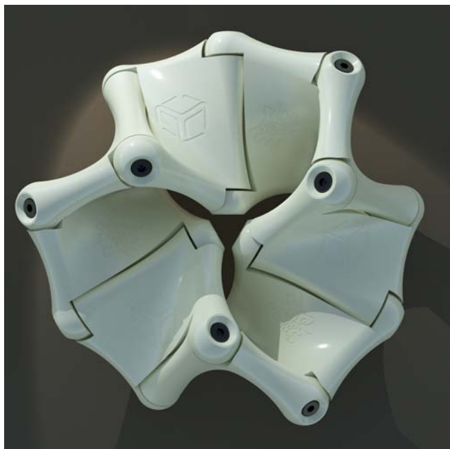
Fig. 1. Rendering of a nine-hinged Möbius kaleidocycle (MK9) made from nine identical links connected through revolute hinges. This ring linkage has only a single degree of freedom manifested by a cyclic everting motion ( Movie S1 ).
