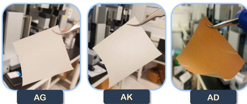
Figure 1. Commercial polyamide TFC membranes used in this study: Veolia AG and Veolia AK, which are standard and low-pressure brackish water reverse osmosis membranes, and Veolia AD, which is designed for delivering high NaCl rejection under seawater operating conditions.
