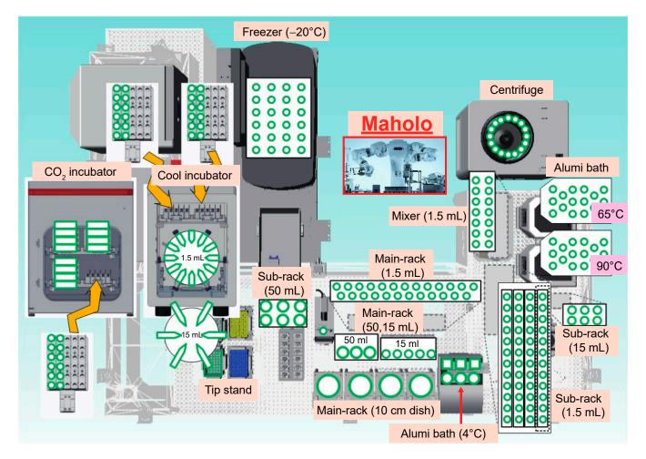
**Figure 4.** General arrangement drawing for the experimental devices placed around the Maholo. The Maholo is centrally located. Note that the magnetic stand and the refrigerated centrifuge are located in the middle and upper right corner, respectively.
