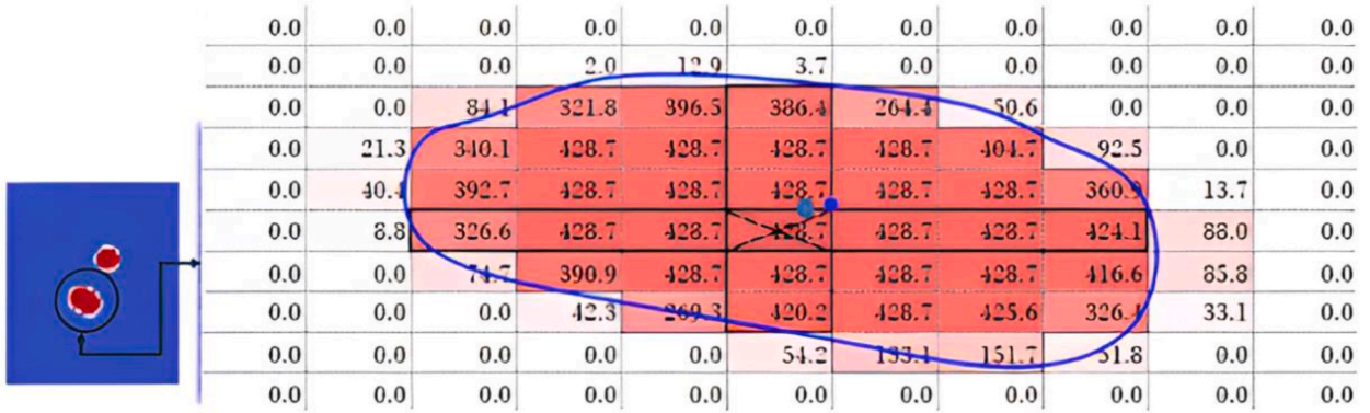
Fig. 7. Cross section area of a cerebral vessel processed by the smoothing algorithm: starting from the central axis points previously identified, located at the center of the corresponding voxel, highlighted in the yellow box, the adjacent voxel elements located along the x and y direction, marked in the blue area, are counted in computing the new central points coordinates, based on a weighted average. The procedure iterates in the remaining other directions in order to provide the new central point location, suitably smoothed.
