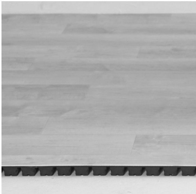
Figure 1 The MM-flooring. Newly developed flooring material with a mechanical metamaterial structure (MM-flooring). MM-flooring, mechanical metamaterial flooring.
