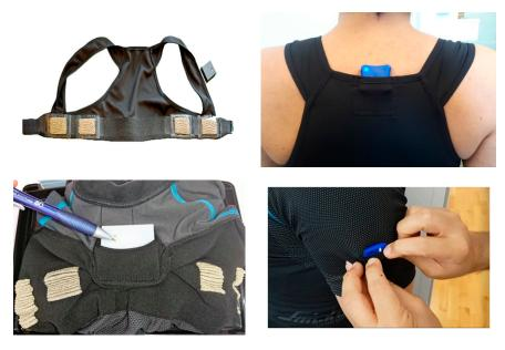
Figure 2. Vest (top) and t-shirt (bottom), including textrodes and ECGZ2 and IMUs.
