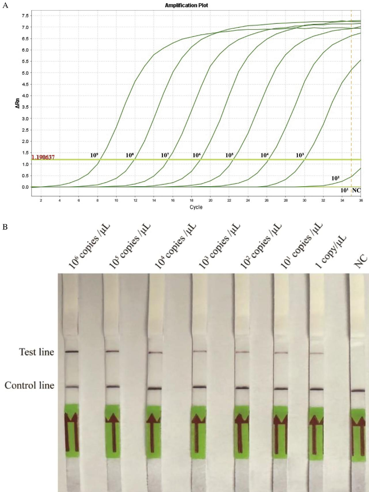
**Fig. 5.** Sensitivity of the RPA-CRISPR/Cas13a assay for *V. parahaemolyticus* detection. A. TaqMan-qPCR method; B. RPA-CRISPR/Cas13a-LFD method. NC, negative control.
