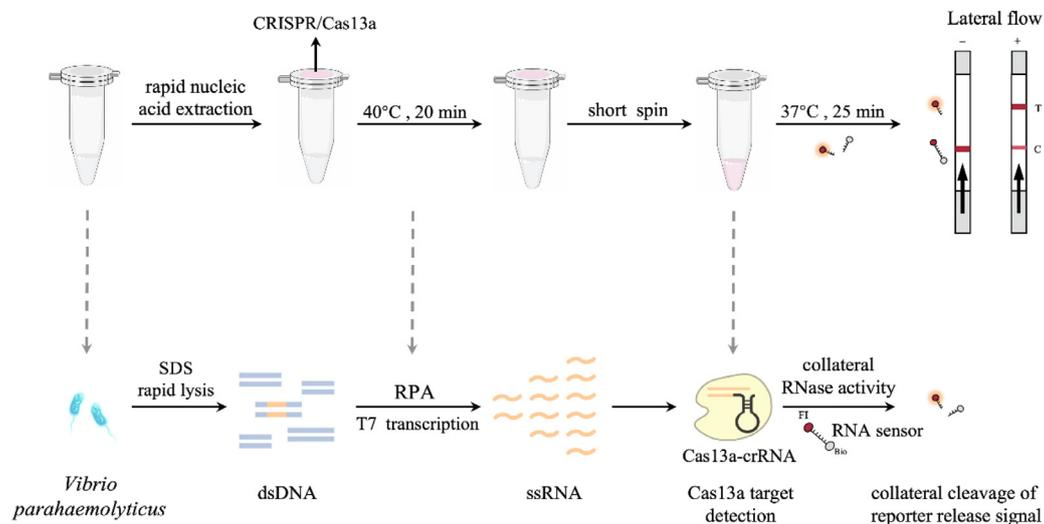
Fig. 1. RPA-CRISPR/Cas13a method for the detection of *V. parahaemolyticus*.
