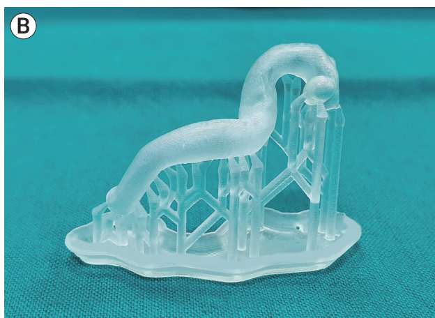
Fig. 5. (A, B) A 3D hollow model of a patient's blood vessel regions of interest, created using a 3D printer.
