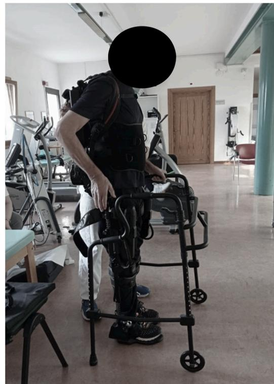
**Fig. 1.** Subject wearing the overground wearable exoskeleton during the robotic gait training.
