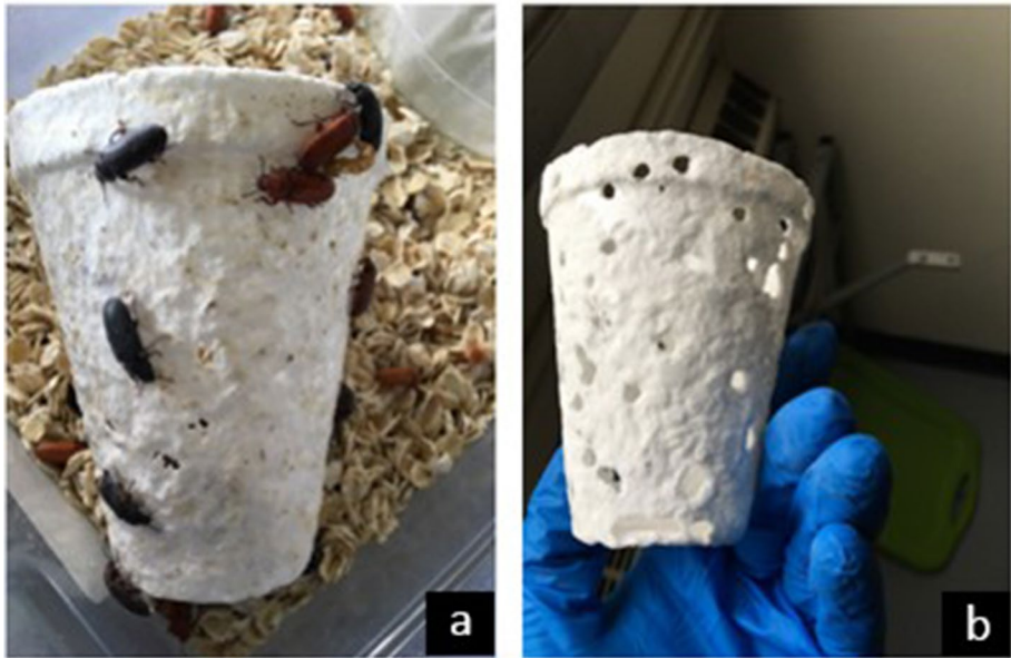
Fig. 2 a EPS cup consumed by beetles. b EPS cup consumed by mealworms. These studies were conducted in a regulated lab
