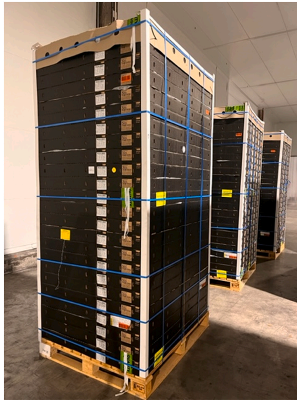
Fig. 3. Neon yellow and neon green stickers showing the locations of sensors in the pallets.
