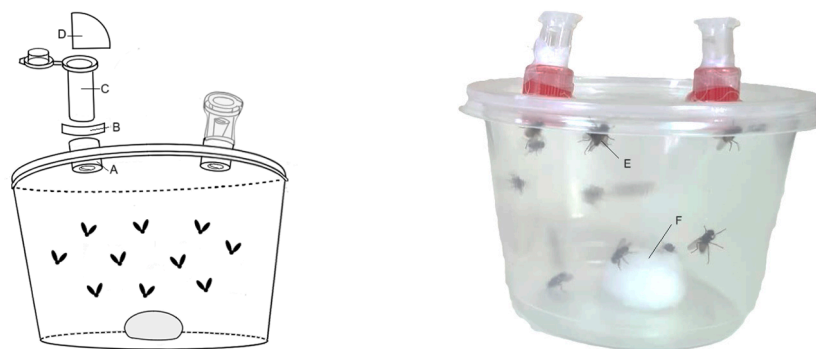
Figure 1. Outline of the components of the fumigant test device, showing the sample test tube lid (A), the tulle mesh (B), the Eppendorf tube (C), the filter paper (D), adult flies (E), and moistened cotton swab (F).
