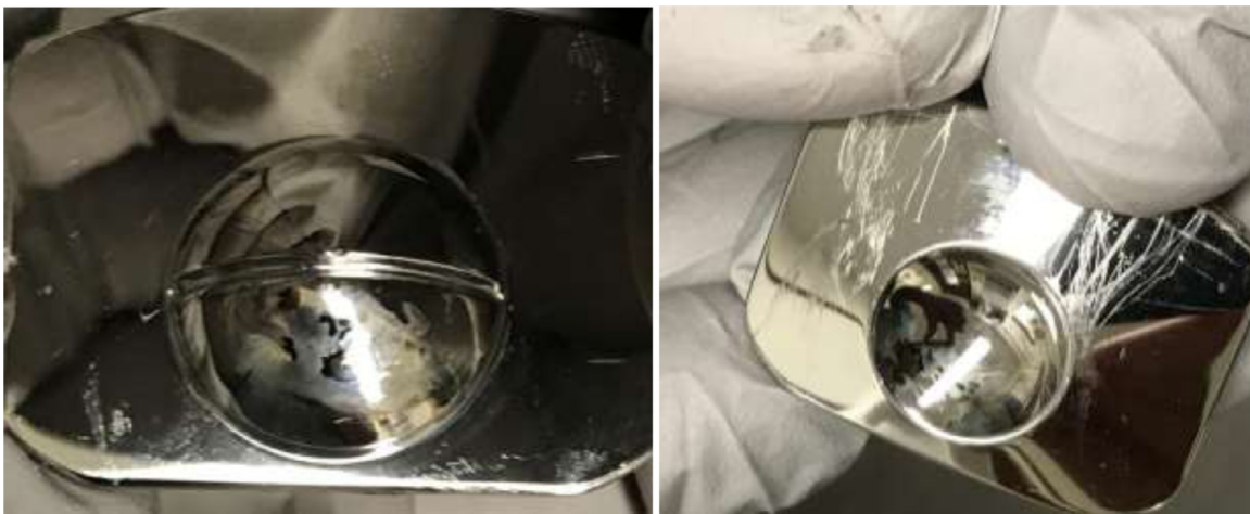
Fig. 8. Total disc replacement (TDR) implants showing signs of wear.
