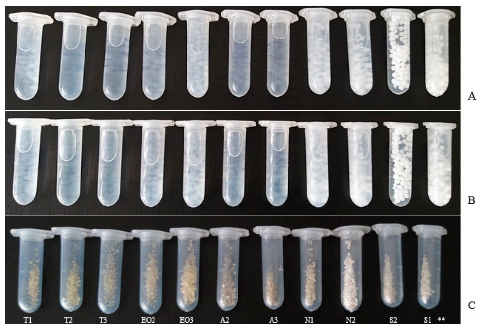
Figure 5. NEO-loaded microcapsules. Wet capsules in the crosslinker solution: (A) 2% solution; (B) 5%; (C) dry microcapsules (2% crosslinker solution). ** The code of microcapsules is given in Table 1.
