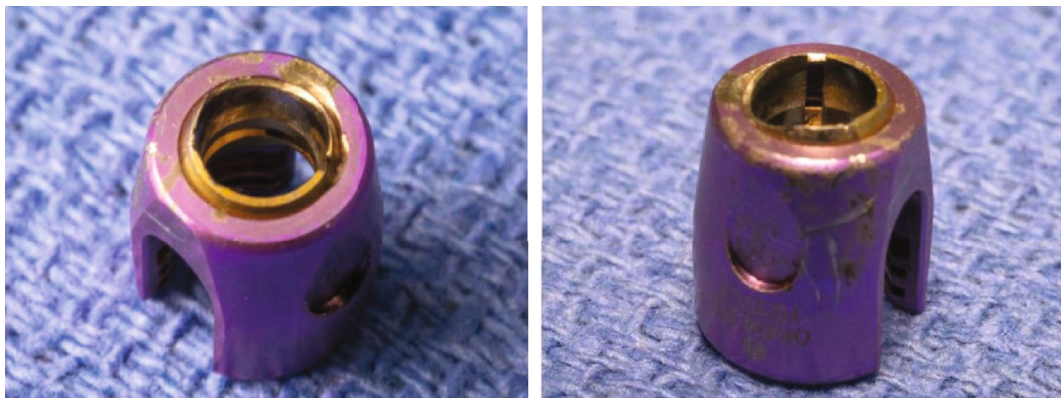
FIGURE 3: Erosion of the coupling portion of the tulip head from motion at the tulip-screw junction.
