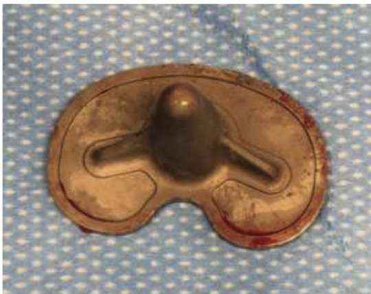
Figure 1. Intraoperatively removed debonded tibial component.
