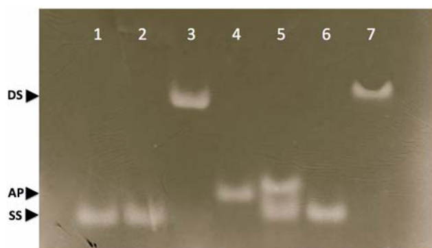
Figure 4. 20% Native-PAGE experiment illustrating differing duplex-forming abilities with T0 between strands S0, S2-A, and S2-AP: lane 1, S0; lane 2, T0; lane 3, S0 + T0; lane 4, S2-AP; lane 5, S2-AP + T0; lane 6, S2-A; lane 7, S2-A + T0. Conditions: 25 mM NaCl, 1 \times TB, 24 h at 100 V, 293 K.
