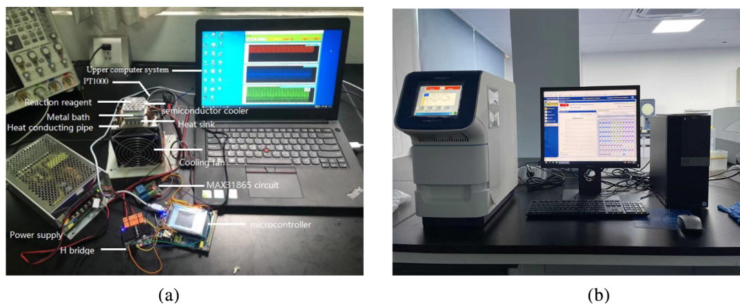
Figure 5. Experimental PCR system and device. (a) Designed PCR system and (b) commercial qPCR instrument.
