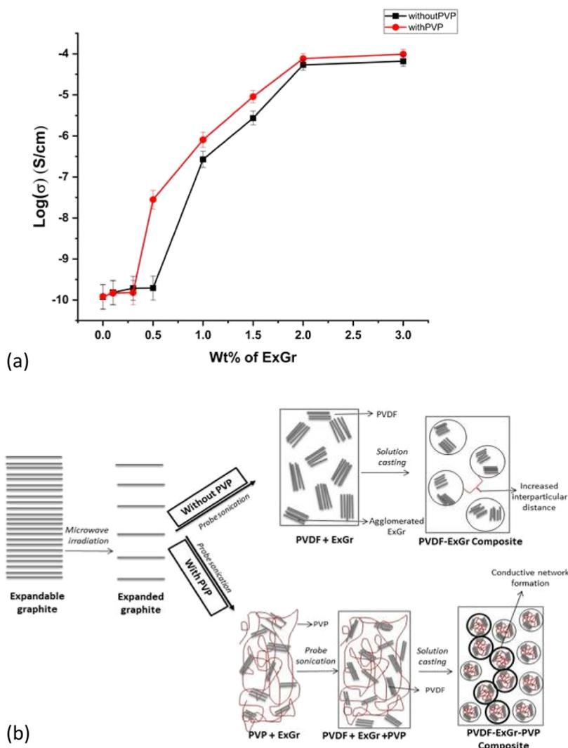
**Figure 1.** (a) Variation of electrical conductivity in the solvent-cast PVDF-ExGr nanocomposite films with and without PVP. (b) Model depicting the conducting network formation in the PVDF ExGr composites without and with PVP.
