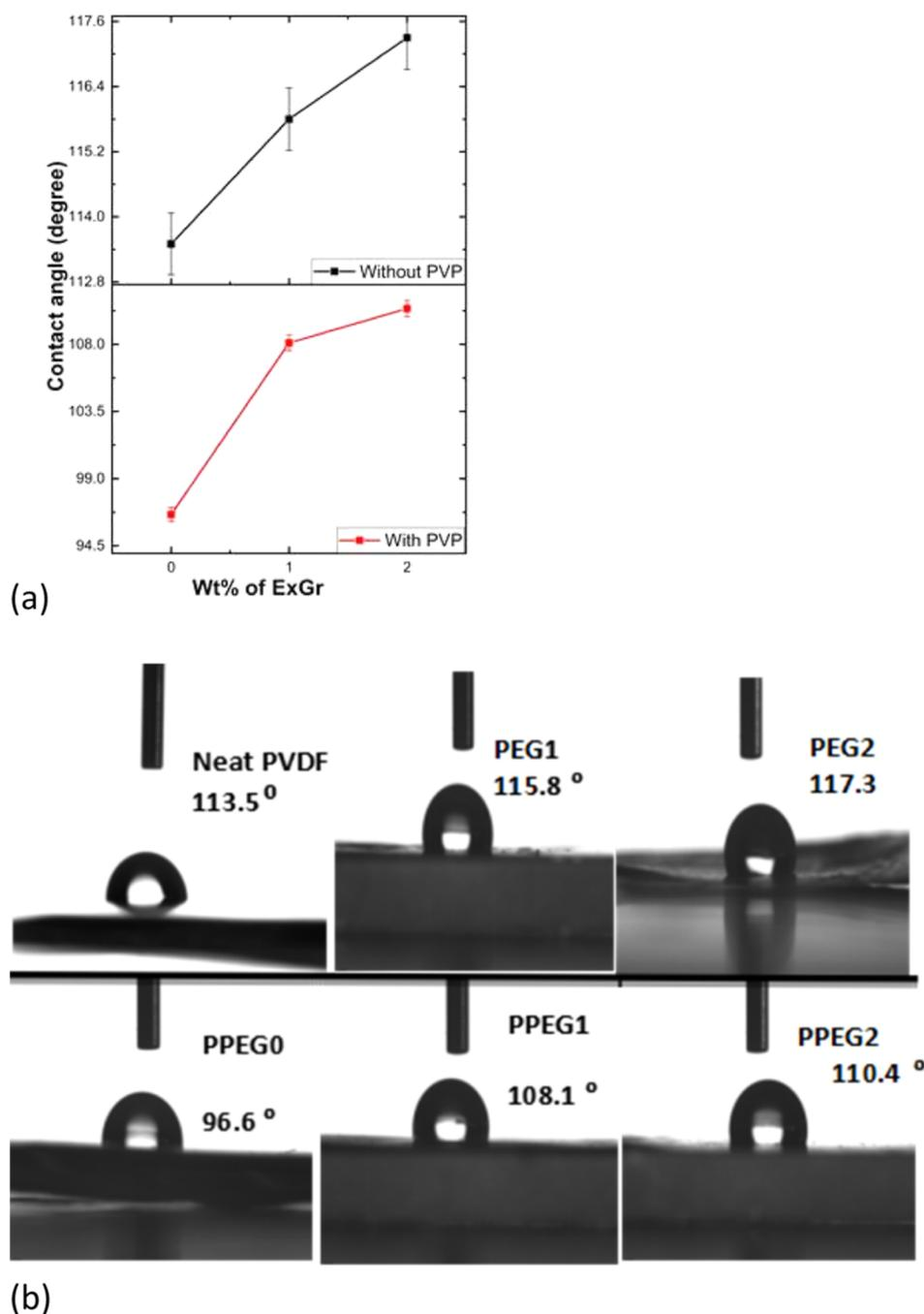
**Figure 8.** (a) Variation of contact angles of solution-blended PVDF- $x$  wt % ExGr ( $x = 0, 1, 2$ ) without and with 1 wt % PVP vs ExGr loading. (b) Digital pictures depicting contact angles of solvent-cast samples: (from top left) neat PVDF, PEG1, PEG2, PPEG0, PPEG1, and PPEG2 composite films.
