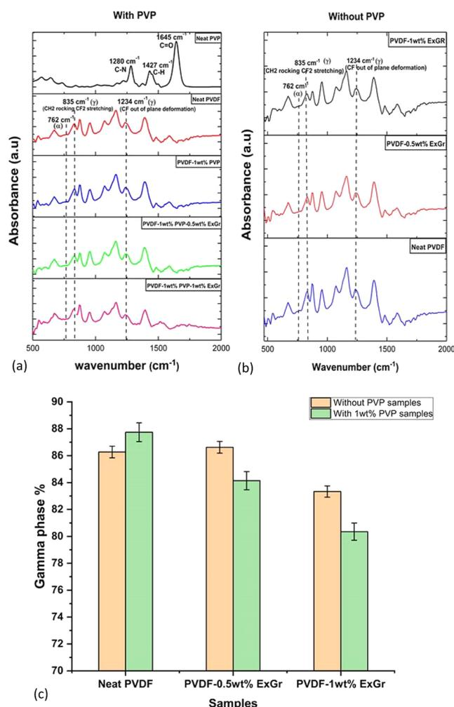
**Figure 5.** FTIR of spectra of solvent-cast samples (a) with PVP (neat PVP, neat PVDF, PPEG0, PPEG0.5, PPEG1) and (b) without PVP (neat PVDF, PEG0.5, PEG1). (c) Electroactive gamma phase content in the solution-blended PVDF-ExGr nanocomposite film with and without 1 wt % PVP.
