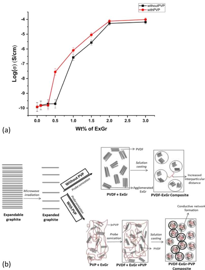
**Figure 1.** (a) Variation of electrical conductivity in the solvent-cast PVDF-ExGr nanocomposite films with and without PVP. (b) Model depicting the conducting network formation in the PVDF ExGr composites without and with PVP.
