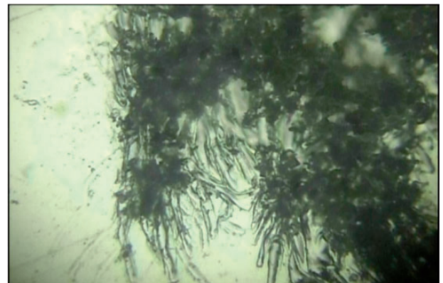
Fig. 7. Damage (punctures) due to R. dominica . Polypropylene packaging with thickness 0.04 mm.
