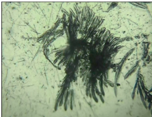
Fig. 4. Damage (punctures) due to R. dominica . PE packaging with thickness 0.04 mm.
