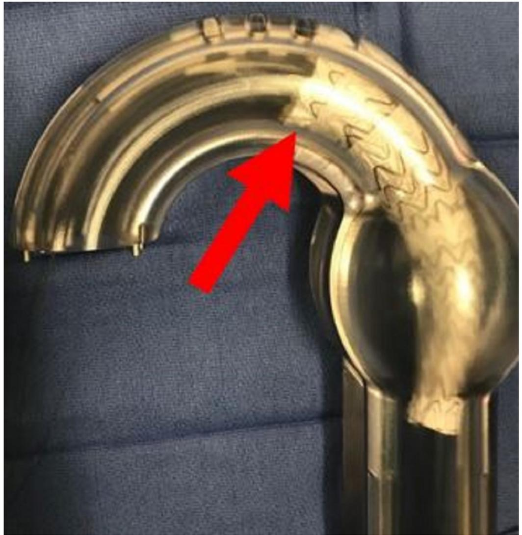
**FIGURE 10: Aortic glass model with deployment of the final thoracic aortic graft (red arrow).**
