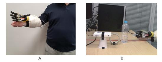
**Figure 3.** The pick-and-place experiment setup. (**A**) The participant wore the Robo-limb prosthetic hand on his right arm with a customised socket. The prosthetic hand was powered by the battery mounted on the socket and the Arduino system was connected to the computer so that the user could switch the controller during use through the user interface. (**B**) The participant was instructed to grasp and relocate three objects using the prosthetic hand.
