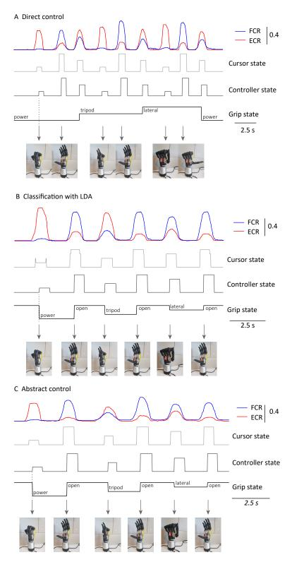
Figure 4. Control signals for the (A) direct controller, (B) linear discriminant analysis (LDA) classifier, and (C) abstract controller.
