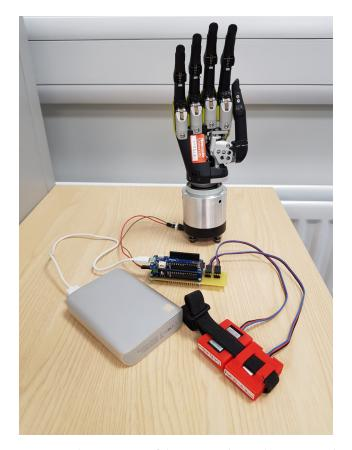
Figure 1. The prototype of the proposed myoelectric control system.
