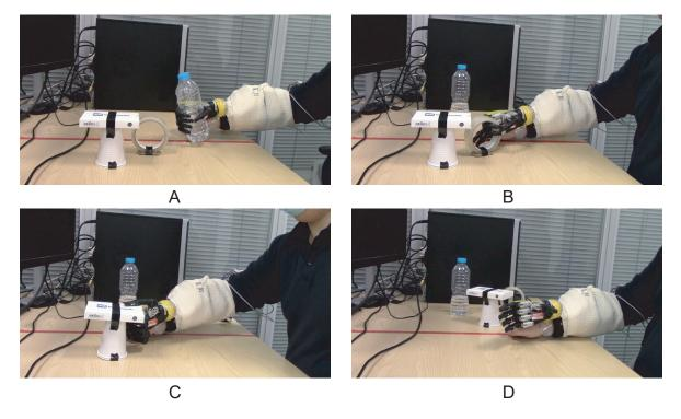
**Figure 5.** Real-time pick-and-place experiment with three different control algorithms. The participant (**A**) lifted the bottle with a power grip, (**B**) lifted the roll of tape with a tripod grip, (**C**) lifted the credit card simulator with a lateral grip, and (**D**) opened the prosthetic hand to relocate the objects.
