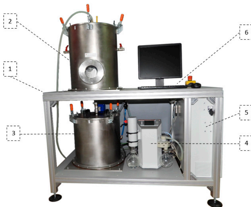
Figure 2. The intensified heat transfer adsorption bed (IHTAB) facility: 1—aluminum frame, 2—reaction chamber, 3—evaporator chamber, 4—vacuum pump, 5—data acquisition and control system, 6—computer.
