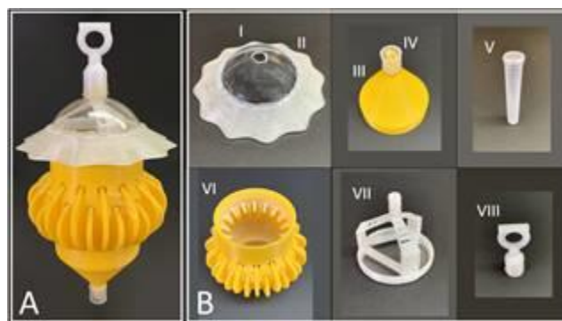
Figure 1. Stem trap. (A) Assembled stem trap used for the study. (B) Parts of the stem trap: I. Semi-circular, clear, plastic dome with an aperture at the top; II. Rain skirt; III. Funnel structure; IV. Funnel outlet for connecting the cap of the capture vial; V. Capture vial; VI. Body of the trap with stem-like protrusions on the outer surface leads to entry holes to guide ACPs into the trap's interior; VII. Tripod structure; and VIII. Hanging nut used to deploy the trap and connect the tripod structure with the dome.
