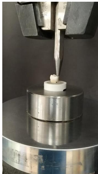
Figure 2. Fracture strength test by universal testing machine using a 3 mm diameter steel ball contacting the restoration at the isthmus area at a crosshead speed of 0.5 mm/min until fracture.
