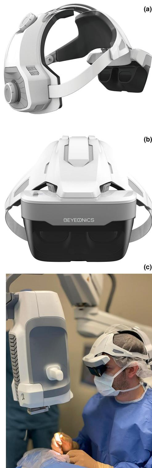
**Fig. 1** Side view (a) and front view (b) of the three-dimensional head-mounted display, and the head-mounted display being used in DSAEK surgery (c)
