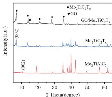
Fig. 3 XRD pattern of GO/Mo<sub>2</sub>TiC<sub>2</sub>T<sub>x</sub>.
