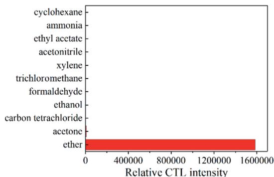
Fig. 9 CTL response of sensor to different compounds.
