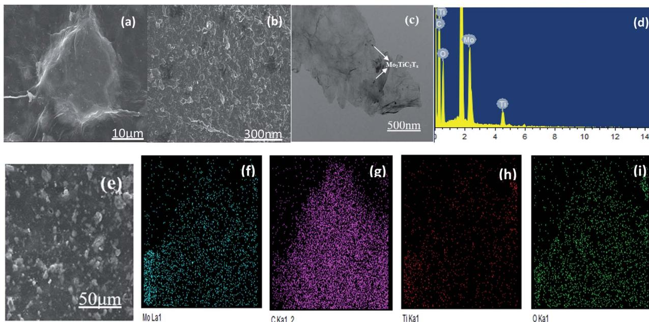
Fig. 2 (a) and (b) SEM, (c) TEM images of GO/Mo<sub>2</sub>TiC<sub>2</sub>T<sub>x</sub>, (d) EDS spectrum of the GO/Mo<sub>2</sub>TiC<sub>2</sub>T<sub>x</sub>, (e)–(i) SEM image and EDS mapping of GO/Mo<sub>2</sub>TiC<sub>2</sub>T<sub>x</sub> catalyst.
