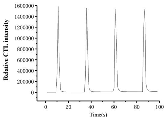
Fig. 5 Typical CTL spectra at optimum conditions. (concentration: 950 ppm; flow rate: 400 mL min<sup>-1</sup>; the temperature: 155 °C.)
