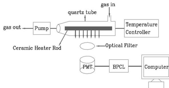
Fig. 1 Schematic diagram of the CTL-based sensor system.
