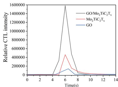
Fig. 4 Comparison of CTL performance of different materials (concentration: 950 ppm; flow rate: 250 mL min<sup>-1</sup>; temperature: 165 °C).
