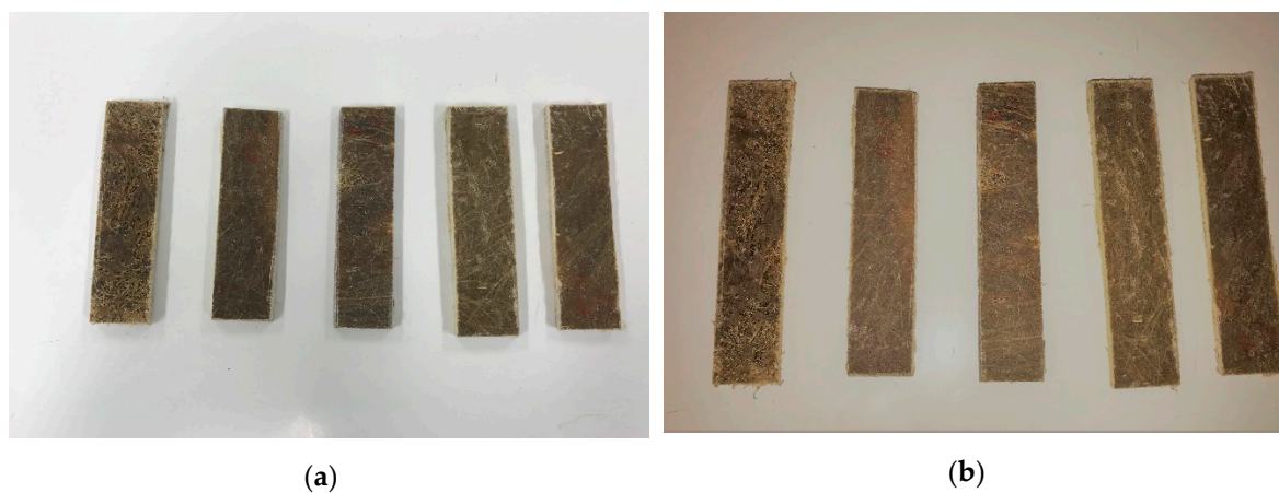
Figure 3. Hemp and flax fiber hybrid composites (a); banana and pineapple fiber hybrid composites (b).
