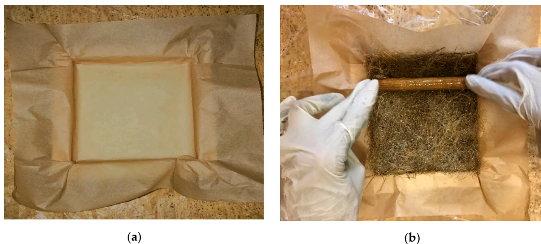
Figure 2. Mold material for fabrication purpose (a); roller on the composite surface (b).
