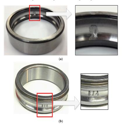
Figure 4. The faulty bearing: (a) outer race fault; (b) inner race fault.
