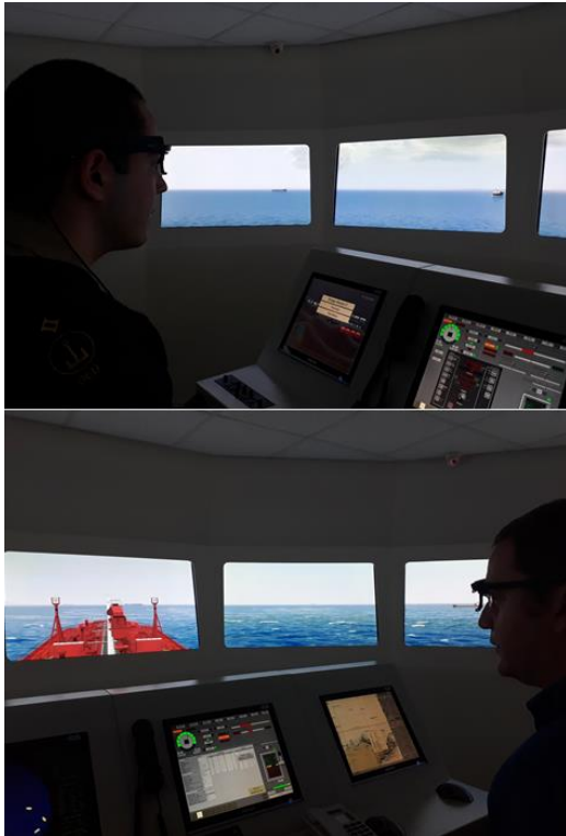
Figure 2. A participant with the eye tracking glasses executing a simulation exercise in the full mission bridge simulator.
