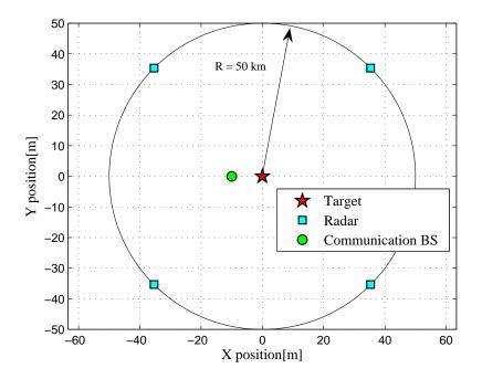
Figure 4. Simulated 2D scenario with locations of multiple radars, communication BS and target.
