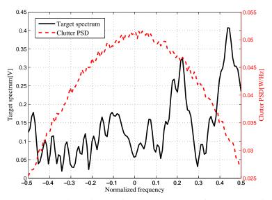
Figure 8. Target and signal-dependent clutter spectra with respect to Radar 4.
