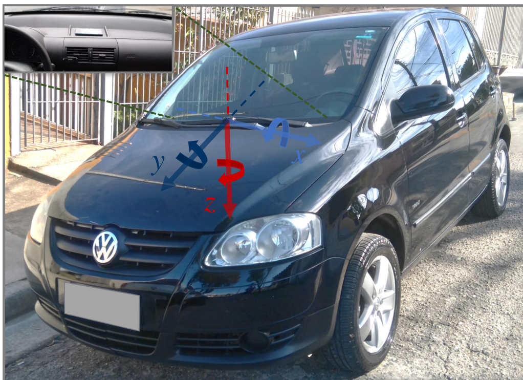
Figure 1. Smartphone installation location (in detail) and coordinate reference system x , y , and z . The x axis points to left and is perpendicular to the vehicle plane of symmetry. The y axis points forward and is parallel to the vehicle plane of symmetry. The z axis extends downwards. The pitch, roll, and yaw are the counterclockwise (right-handed) rotations about the x , y , and z axes, respectively.
