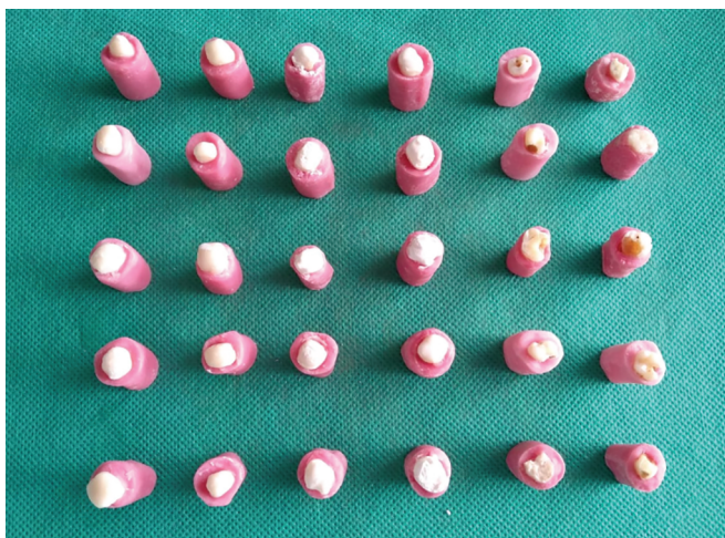
Fig. 1: Tooth specimens embedded in acrylic mould
