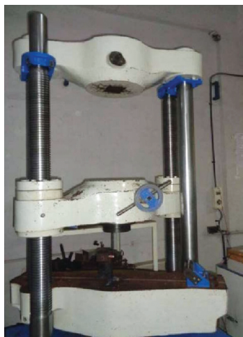
Fig. 4: Universal testing machine: Fine testing machine
