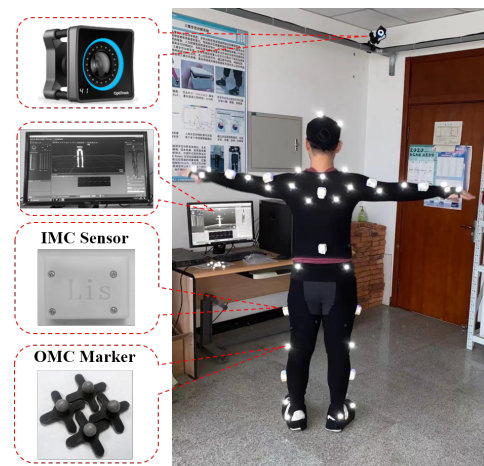
Figure 8. Inertial motion capture (IMC) sensor and optical motion capture (OMC) marker setup shown in the room.
